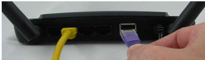
16.) Connect the router's WAN port to your Internet connection (DSL, Cable, Satellite modem, fixed wireless radio, etc.). Wait a few seconds, then see if you can access the Internet from the computer connected to the router. If you can, you're done. If not, see the Troubleshooting section below.
